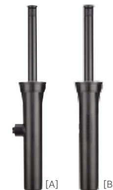
[A] PROS-06-SI [B] PROS-06 Retracted height: 8 3/4" Pop-up height: 6" Exposed diameter: 2 1/4" Inlet size: 1/2"
