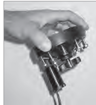
Diaphragm support ring prevents stress failures.
